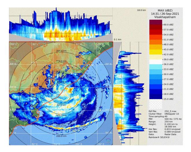
Reflectivity imagery from Doppler weather RADAR Vishakhapatnam based on 2000 hrs IST of 26<sup>th</sup> September 2021.
